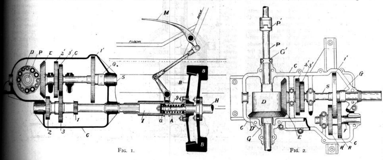
bevel gear E, which is in constant mesh with the gear D' attached to the end of the differential D, thus driving the countershaft P. (See Fig. 2.) Ball thrust bearings G and G G are fitted to take up the end thrust.
